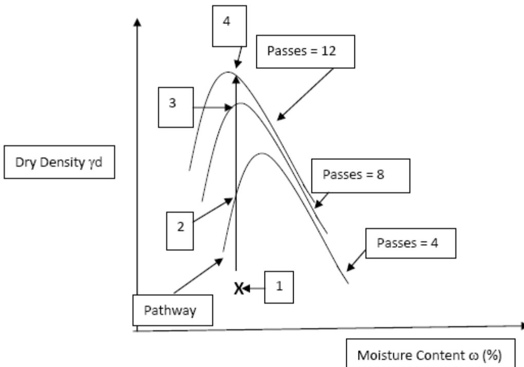
**Figure 3 - Compaction with the Same Compactor and Moisture Content to Achieve Higher Densities**
