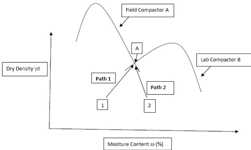
**Figure 1 - Compacted Soil Properties Depend on the Energy/Stress Path of Compaction**
